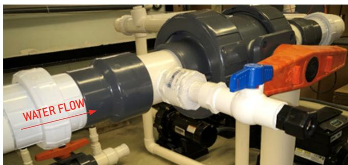
Inlet water pitot tube - notch facing downstream
