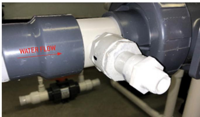
Inlet water pitot tube – notch facing upstream
